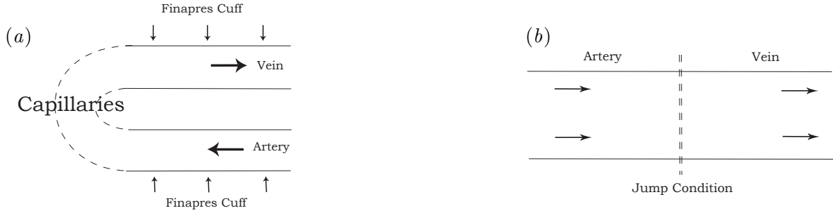
FIGURE 8: (a) An idealised sketch of the Finapres and artery system. (b) A simplified system, replacing the capillaries with a jump condition. The Finapres exerts compression on both the vein and the artery.
