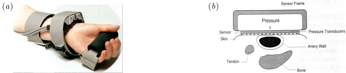
FIGURE 2: The Colin Radial Artery Tonometer. (a) A photograph of the device in operation. The pressure transducers are located in the central block, and the straps at either end are part of a separate splint designed to keep the wrist still. (b) A cross-section of the wrist showing how the device works.
